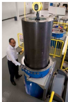
Volant fibre carbone 1 tonne 8000 – 16 000 tr/min
