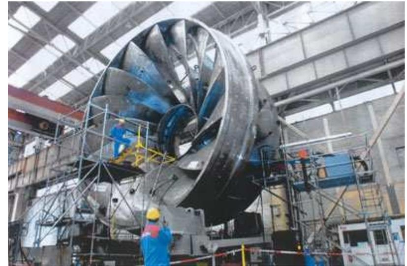
Turbine Neyrpic 700 MW, Ø 9.8 m, 425 t, 75 tr/min
