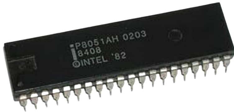
8051 Intel CPU (1980) CPU only, not a MCU
