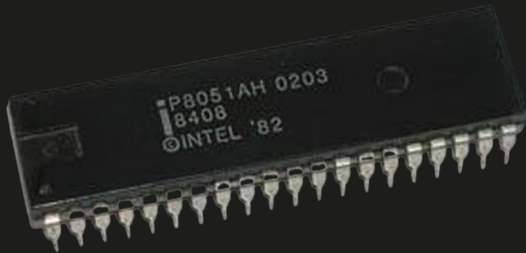
8051 Intel CPU (1980) CPU only, not a MCU
