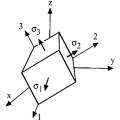
$$\sigma = \begin{bmatrix} \sigma_{xx} & \sigma_{xy} & \sigma_{xz} \\ \sigma_{yx} & \sigma_{yy} & \sigma_{yz} \\ \sigma_{zx} & \sigma_{zy} & \sigma_{zz} \end{bmatrix} (\vec{x}, \vec{y}, \vec{z})$$
