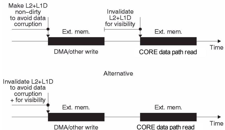
**Figure B-2 External Memory: DMA Write, CORE Read (Code)**
