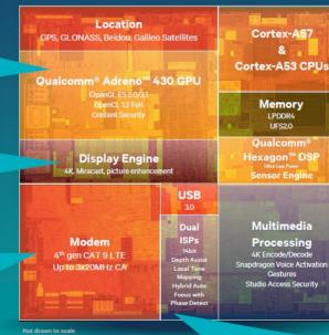
Qualcomm Technologies' FIRST 14-bit Dual ISP for highest quality, depth enabled photography. Up to 21MP for main camera with depth assist, phase detect, for sharper dual camera user experiences FIRST Announced ARM®v8-A/64-bit using Cortex®-A57+ Cortex®-A53
