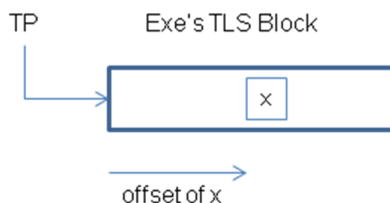
Figure 7. Static Executable TLS Run-Time Representation
